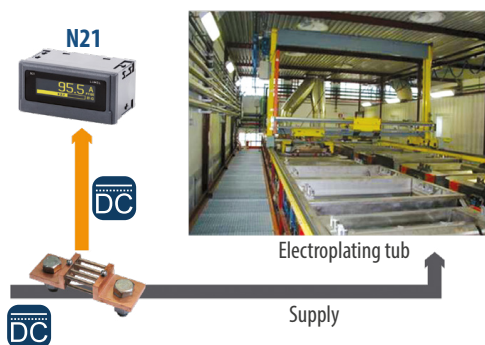
CURRENT MEASUREMENT IN AN ELECTROPLATING PLANT
