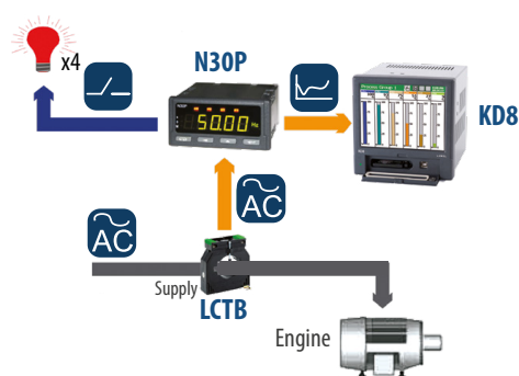
MEASUREMENT, ALARMING AND LOGGING OF LOAD CURRENT FOR A 1-PHASE ENGINE
